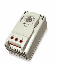
Type of material: Standard colour: Protection degree: Mounting on: Fixing system: Electrical connection: Electrical section wires: Sensing element type: Setting/indexing: Operating temperature: Storage temperature: External dimensions: Approvals: PC/ABS Gray RAL 7035 IP20 DIN rail 35 mm (EN 50022) snap-on Screw terminals From 0.75 mm² to 4.0 mm² Polyamide ribbon External knob and screw driver / 10% From 10 to 40°C From -20 to +50°C 94x54x52 mm CE; cURus certified till max 80% RH
