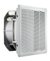
FF series exhaust filter and filter fans represents a side-mounted cooling solution with filtered ambient air to maintain optimum ventilation inside the electrical cabinets. Screwless connection, fast tool-free mounting system with clip and maintenance friendliness are the main benefits. Available in a wide range of configurations for both indoor and outdoor use.
