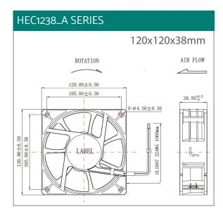
**Casing Material:** Thermoplastic UL 94V-0/Black **Impeller Material:** Thermoplastic UL 94V-0/Black
