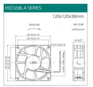
Casing Material: Impeller Material: Motor Protection: Rotation: Storage Temperature: Operating Temperature: Lifetime (L10 at 40°C): Electrical Connection: Bearings: Safety Approvals: Thermoplastic UL 94V-0/Black Thermoplastic UL 94V-0/Black Locked Rotor Protected Clockwise (from label side) -40°C to +70°C -30°C to +70°C 70,000hrs 2x Lead Wires 2x Ball Bearings CE, ATEX
