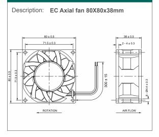
Casing material: Impeller material Protection degree: Fixing system: Motor protection: Storage temperature: Rated temperature range: Lifetime L10 at 25°C: Electrical connection: Approvals: Weight: Thermoplastic in black color, UL 94 V-0 Thermoplastic in black color, UL 94 V-0 IP20, according to EN 60529 standard by No 4 M4 screws Impedance From -40°C to +80°C From -10°C to +70°C 50,000 h 2 leads 24 AWG UL1430 CE 0.270 kg
