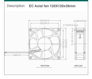
Casing material: Impeller material Protection degree: Fixing system: Motor protection: Storage temperature: Rated temperature range: Lifetime L10 at 40°C: Electrical connection: Approvals: Weight: Thermoplastic in black color, UL 94 V-0 Thermoplastic in black color, UL 94 V-0 IP20, according to EN 60529 standard by No 4 M4 screws Impedance from -40°C to +75°C from -30°C to +70°C ball bearing 50,000 h 2 leads 24 AWG UL1430 CE 0.270 kg
