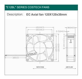
Thermoplastic in black color, UL 94 V-0 Casing material: Impeller material Thermoplastic in black color, UL 94 V-0 Protection degree: IP20, according to EN 60529 standard
