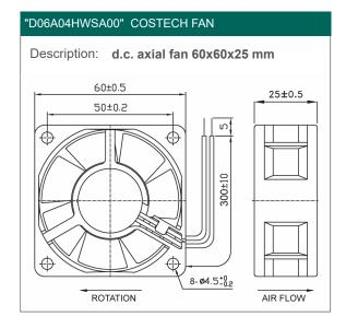
Casing material: Black fibreglass reiforced plastic (PBT) UL
