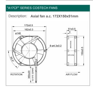
Casing material:Black warnished aluminum UL 94V-0Impeller materialBlack fibreglass reinforced plastic (PBT PC)
