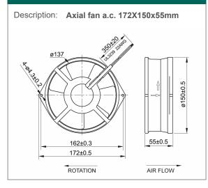
Casing material: Impeller material Protection degree: Fixing system: Insulation class: Motor protection: Storage temperature: Rated temperature range: Lifetime L10 at 40°C: Electrical connection: Approvals: Weight: Black warnished aluminum Metal IP44, according to EN 60529 standard by No 2 M4 screws F thermal from -40°C to +90°C from -40°C to +90°C 40,000 h 2 leads 22AWG UL 3239, 350 mm long UL E223195 1.1 kg
