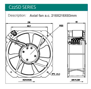
Impeller material:fibre reinforced plastic (PA66) bladesCasing material:aluminium alloy die casting UNI5076
