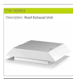
Type of material: Standard colour: Protection degree: Fixing method: Plate thickness: Storage temperature: Lifetime L10 at 40°C: Motor protection: Electrical connection: Earth connection: Appliance class: Weight: Approvals: epoxy painted steel casing RAL 7032 and RAL 7035 IP23, according to EN 60529 standard By No 4 M6 screws any from -20°C to +60°C 50,000 h thermal by 3 core 1.0 mm<sup>2</sup> cable by yellow/green conductor class I 5.29 Kg CE
