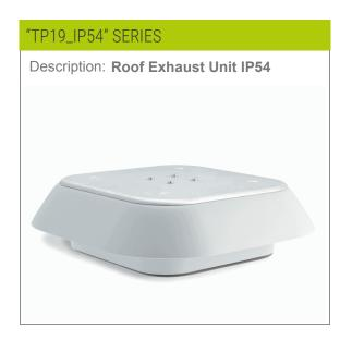
Type of material: ABS/PC alloy and aluminium Standard colour: RAL 7035 - other colours on request Protection degree: IP54, according to EN 60529 standard Fixing method: By No 8 Ø4x16 mm screws for thermoplastic
